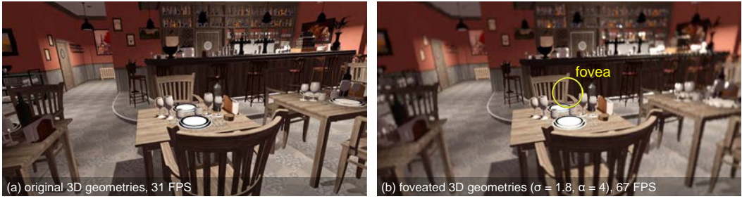
Fig. 11. Comparison of (a) full-resolution rendering and (b) foveated rendering for 3D meshes involving a geometry pass with 1,020,895 triangles as well as multiple G-buffers at 2560 \times 1440 resolution.
