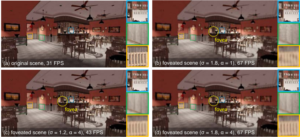
Fig. 1. Results of kernel foveated rendering (KFR): (a) original full-resolution scene rendered at 31 FPS, (b) foveated rendering with \sigma = 1.8 , K(x) = x , rendered at 67 FPS, (c) foveated rendering with \sigma = 1.2 , K(x) = x^4 , rendered at 43 FPS, (d) foveated rendering with \sigma = 1.8 , K(x) = x^4 , rendered at 67 FPS.
