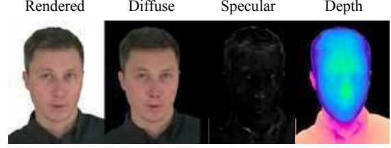
Figure 3. Radiance decomposition. During training, the radiance is modeled using spherical harmonics coefficients, which can be decomposed into diffuse (view-independent) and specular (view-dependent) components. The appearance can be exported as just diffuse or both diffuse and specular texture images.
