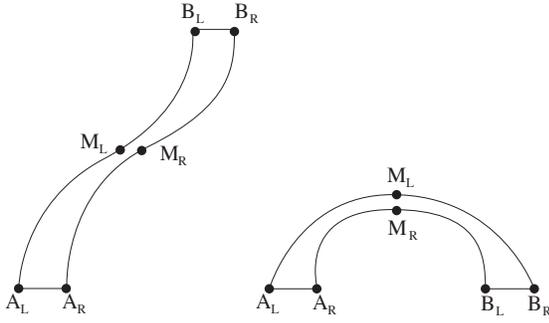
**Figure 4. Control points used in Bézier Curve**
