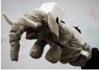
Figure 2: Closer view of an elephant puppet with VRSurus. The elephant puppet wears a custom 3D-printed cap that encapsulates the Arduino microcontroller, an inertial measurement unit and other electronic modules.
