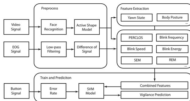
Fig. 1. The proposed vigilance analysis system by combining video and EOG features
